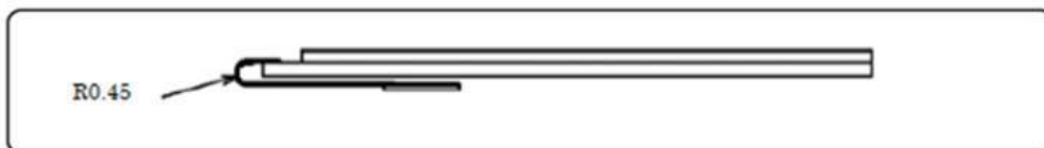
Figure 8-2-1 FPC Bend Specification
