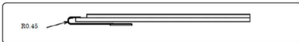
Figure 8-2-1 FPC Bend Specification
