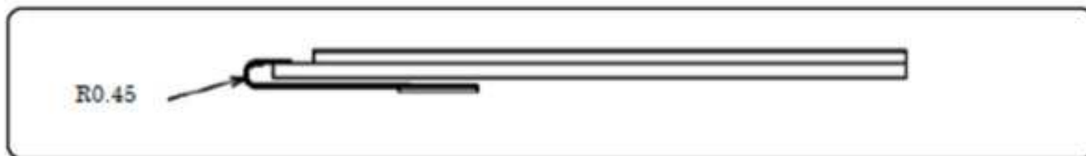
Figure 8-2-1 FPC Bend Specification
