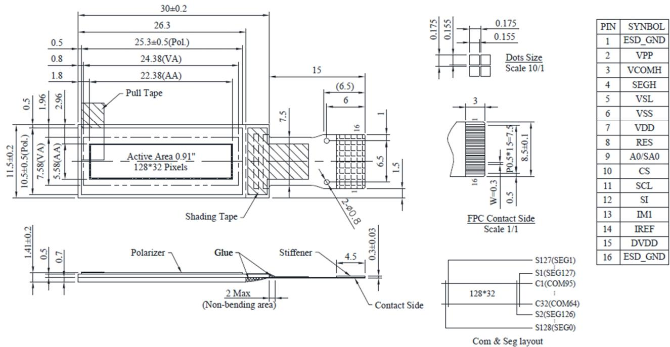
The non-specified tolerance of dimension is  $\pm 0.3\text{mm}$ .
