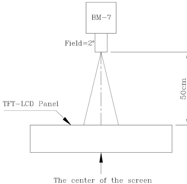
**② The Brightness Test Point Setup**
