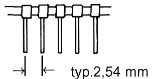
Ø hole in PCB typ. 1,0 mm
